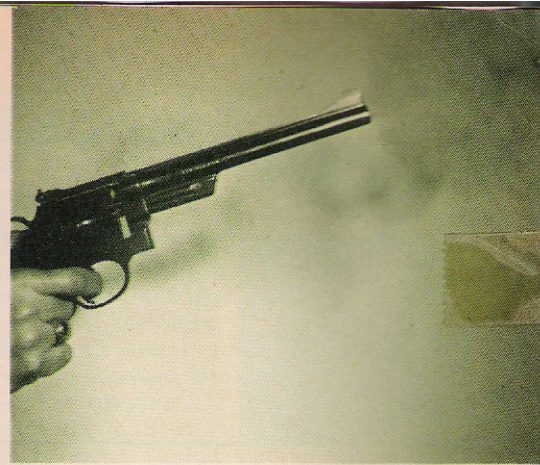
DA revolvers can handle the hottest safe loads, even though there is a fractional gas escape at barrel/cylinder junction.
